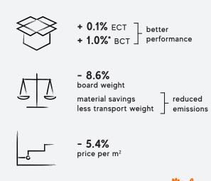
Board grades were simulated using the Mondi Performance simulation tool | Paper price reference taken from EUWID <sup>1</sup> Edge Crush Test | <sup>2</sup> Box Crush Test
