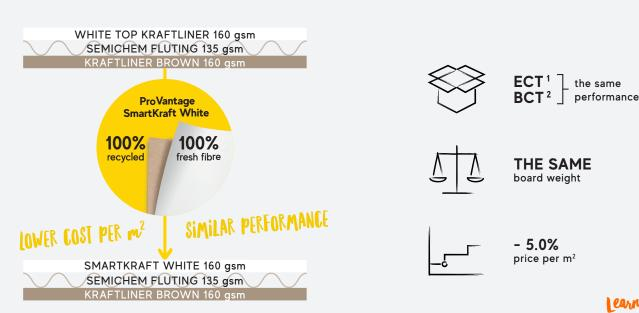
Board grades were simulated using the Mondi Performance simulation tool | Paper price reference taken from EUWID  $^1$  Edge Crush Test |  $^2$  Box Crush Test
