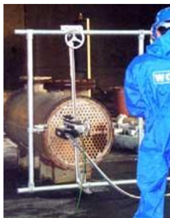
Figure 7: Typical Anti-Withdrawal Device Setup
