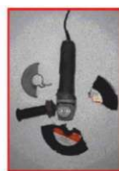
Angle grinder and disintegrated disk
